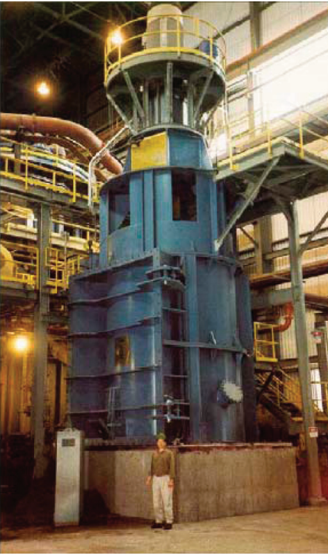
Figure 7a and 7b— These two photographs, printed at approximately the same scale, show the relative sizes of a 3 MW IsaMill relative to a 1 MW tower mill, typically employed in the copper industry for concentrate regrind in larger scale copper-sulphide flotation plants; the unit size impact of high intensity grinding for an IsaMill is clearly seen (extracted from Xstrata Technology presentation given at the IIR Comminution seminar, Perth September 2007)
