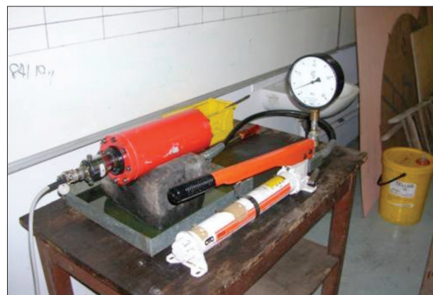
Figure 11—Test apparatus for loading triaxial cells
