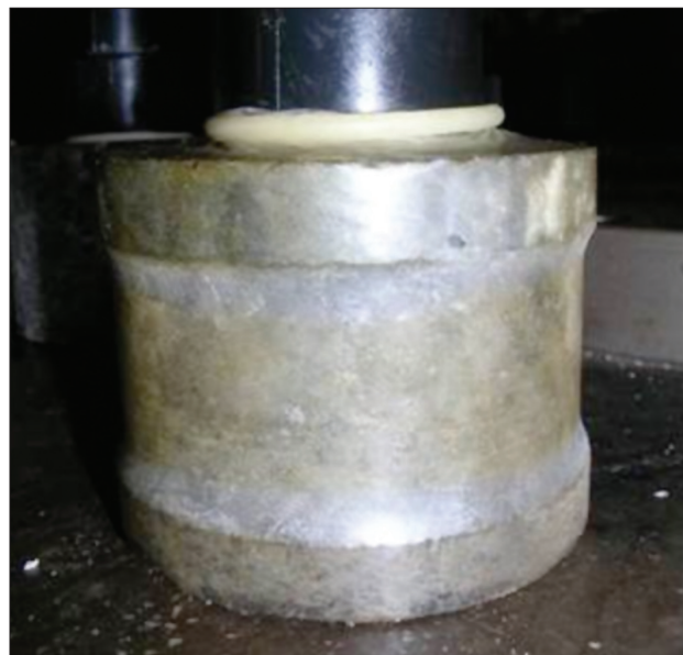
Figure 10—Specially prepared doorstopper sample
