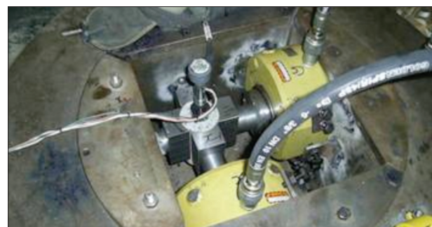
Figure 9—Mechanical biaxial test apparatus for doorstoppers
