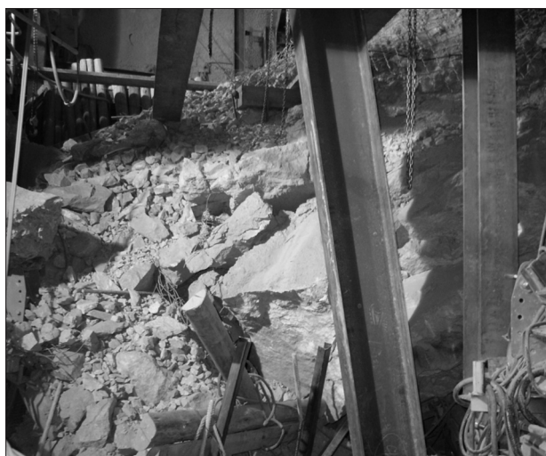
Figure 27—Debris and destruction from the collapse
