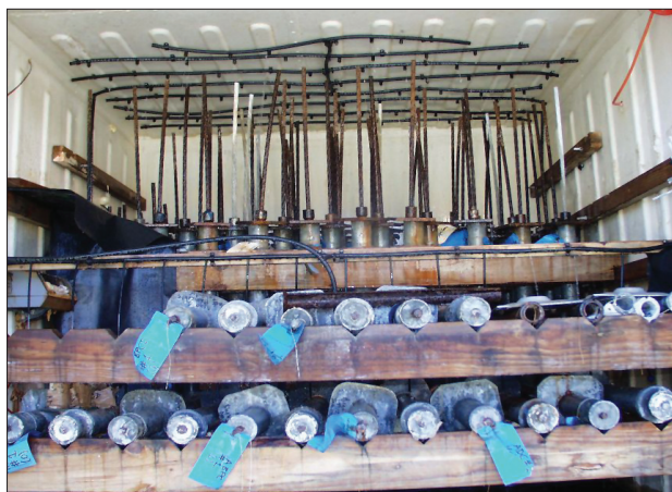
Figure 4—A typical WASM corrosion chamber experiment
