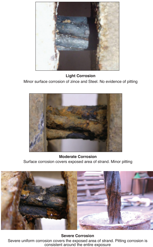
Figure 6—Stages of corrosion damage of cablebolt strand elements
