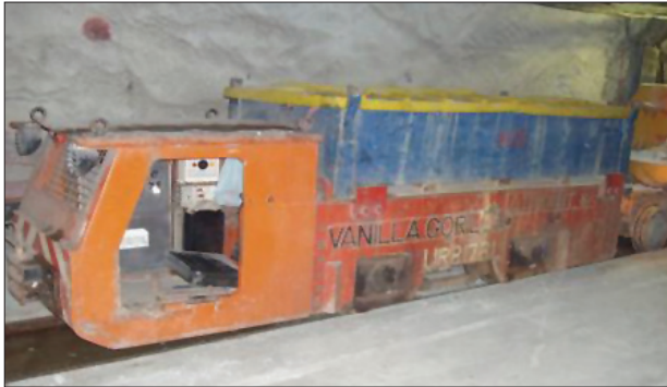
Figure 1—New era Trident 8-ton locomotive
