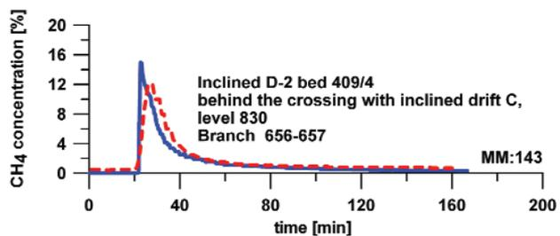
Figure 11—Changes in the concentration of methane, sensor MM:143
