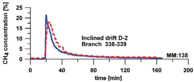
Figure 9—Changes in the concentration of methane, sensor MM:138
