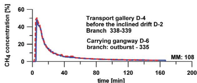
Figure 3—Changes in methane concentration, MM:108 sensor
