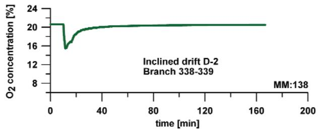
Figure 10—Changes in the concentration of oxygen at sensor next to MM:138
