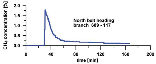
Figure 13—Changes in the concentration of methane, North belt guide, sensor no. 9
