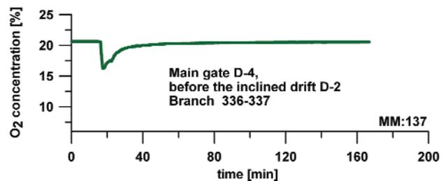
Figure 7—Changes in the concentration of oxygen at sensor next to MM:137
