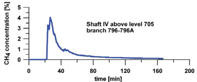
Figure 15—Changes in the concentration of methane, Shaft IV, level 705, sensor no. 11
