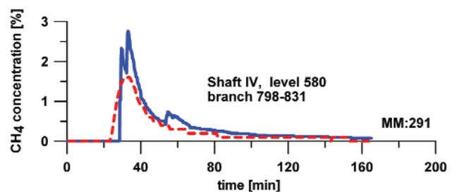
Figure 16—Changes in the concentration of methane, Shaft IV, level 580, sensor MM-291 no. 15
