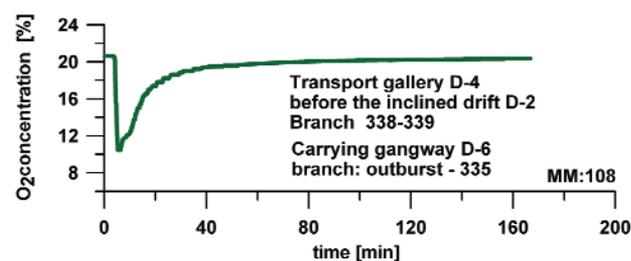
Figure 4—Changes in the concentration of oxygen at sensor next to MM:108
