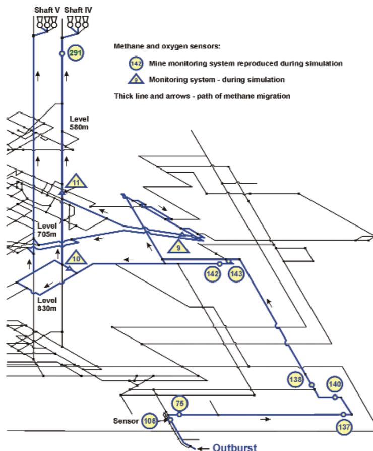
Figure 1—Locations of sensors near section D, bed 409/4
