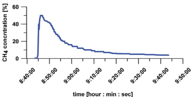
Figure 2—Changes in the concentration of methane, sensor MM-108
