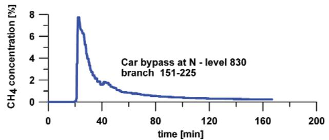
Figure 14—Changes in the concentration of methane, N car bypass, sensor no. 10
