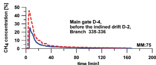
Figure 5—Changes in the concentration of methane, sensor MM:75
