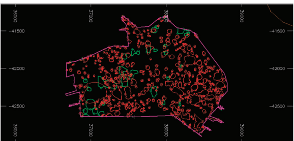
Figure 13—Pothole relationship between Merensky Reef (white circles) and UG2 (grey circles) at Bleskop Shaft
