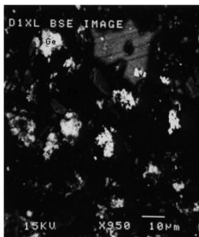
Figure 6—BSE image of a sample of germanium-iron residue
