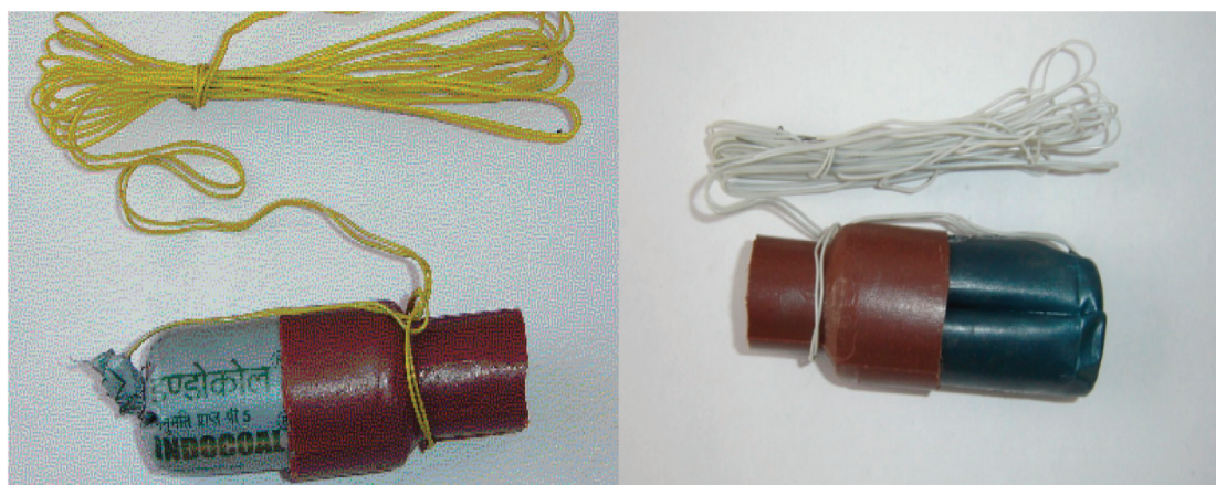
Figure 6—Arrangement for firing explosive with spacer for fume analysis
