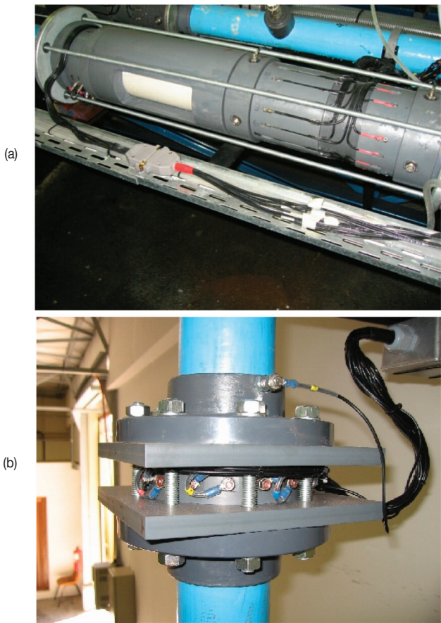
Figure 2—ERT electrode rings in IMST pipe loop: (a) Ø80 mm; (b) Ø80 mm vertical return pipe
