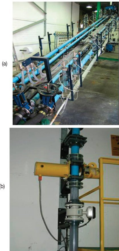
Figure 1 —IMST pipe test loop: (a) the test pipes; (b) flow meter, density gauge and single plane ERT ring in Ø80mm vertical return pipe
