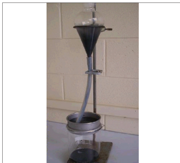
Figure 2—Removing 'sinks' fraction through a clean sieve
