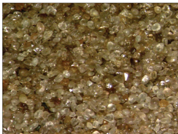
Figure 5—The float fraction of -250+150 \mu\text{m} zircon at 4.25 initial separation relative density
