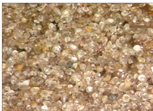
Figure 6—The sink fraction of -250+150 \mu\text{m} zircon at 4.45 initial separation relative density
