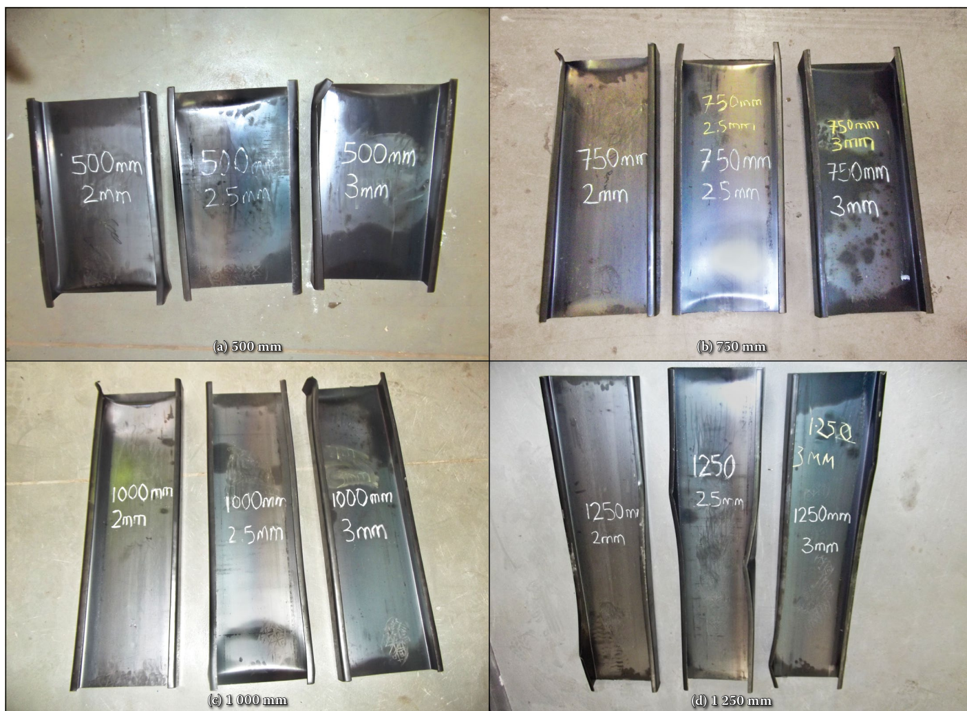
Figure 3 Buckling failure modes
