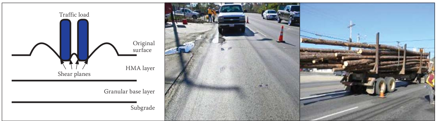
Figure 1 Permanent deformation (PD) of HMA mix (Abdallah & Nazarial 2011)
