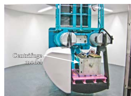
(f) Model in position on centrifuge ready for testing
