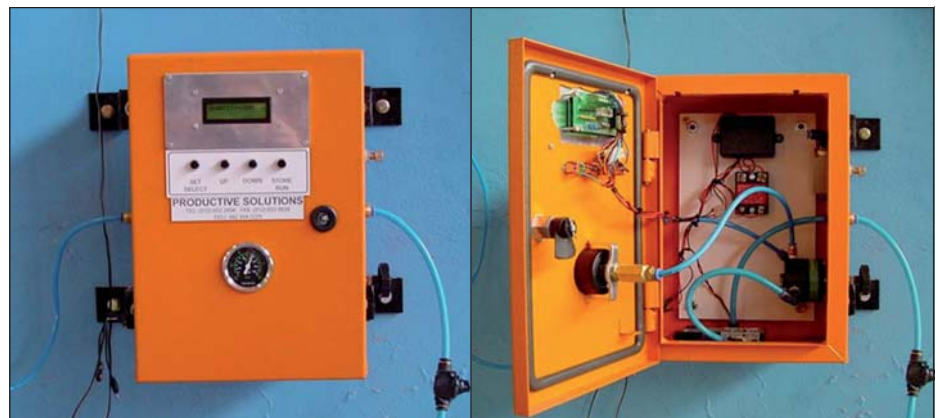
Figure 3: Air Induction Box (AIB) assembly
