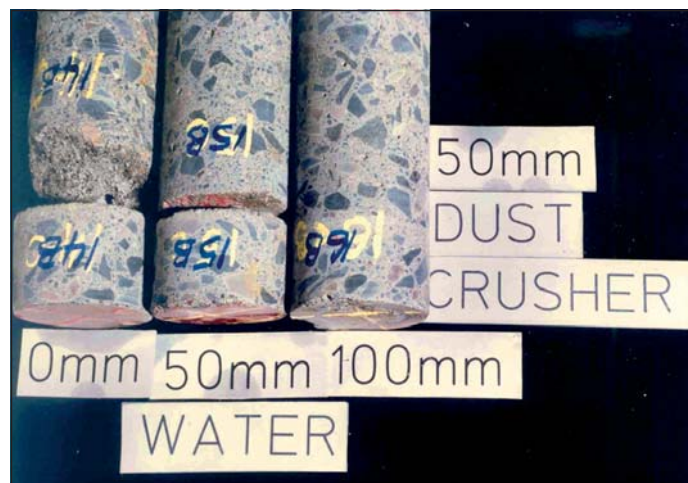
Figure 8 Close-up of contact between “pile” concrete and blinding concrete for “piles” cast with a 50 mm layer of crusher dust at the bottom of the “pile hole”
