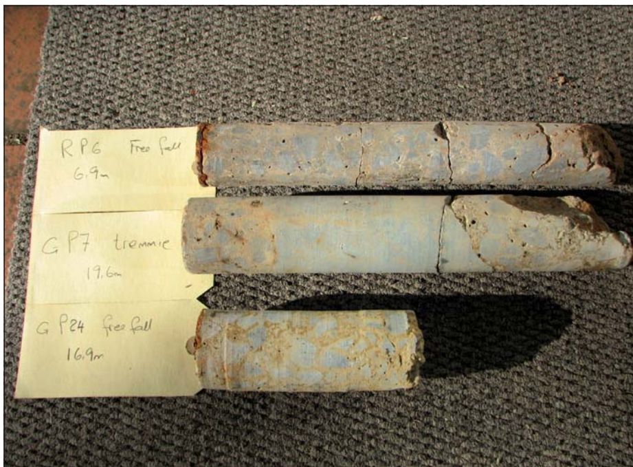
Figure 10 Relative comparison of free-fall and tremie-placed concrete
