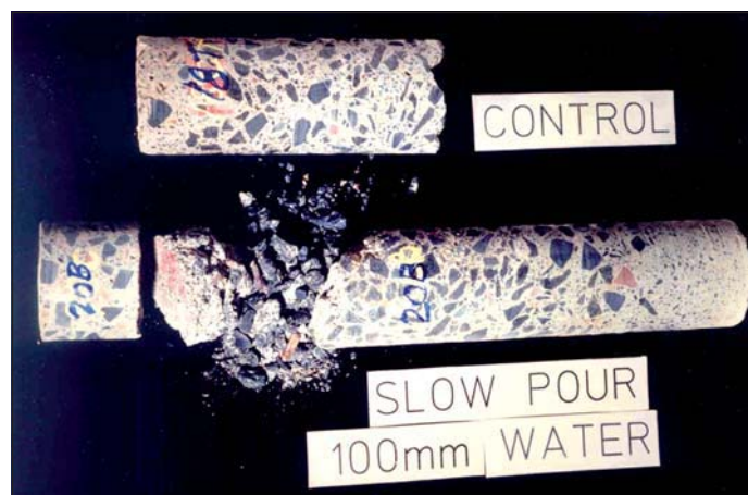
Figure 3 Segregation of concrete poured slowly into 100 mm of water
