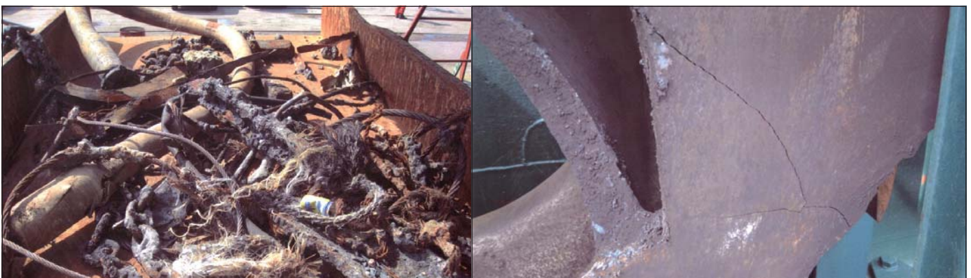
Figure 4 Dredged steel elements and cracked dredger impeller (Photo: Dredging International, April 2010)
