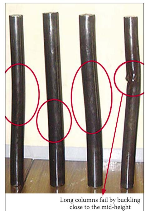
**Figure 3 Photo shows the failure mode of specimen (900 mm long columns)**
