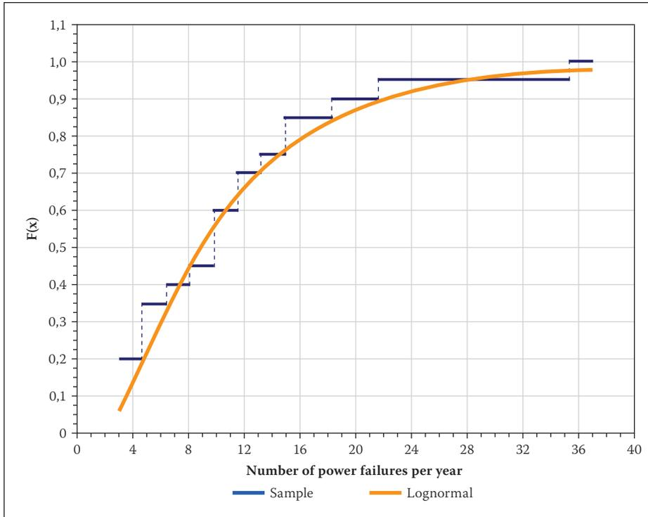
**Figure 4 Number of power failures – cumulative distribution function (Rand Water pump stations)**
