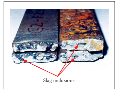
Figure 9 Specimens with slag inclusions
