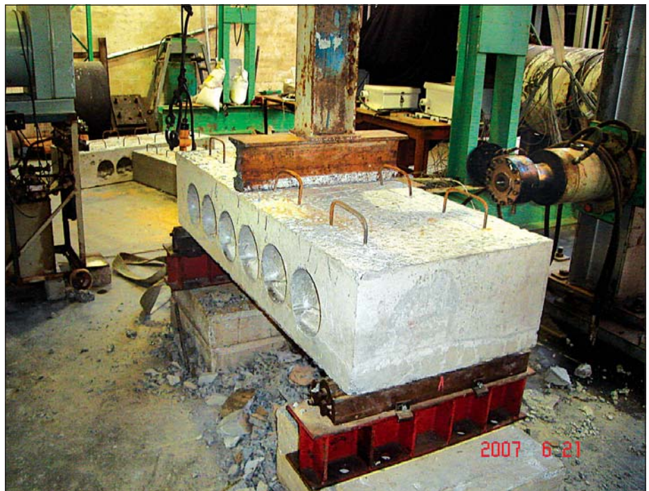
Photo 1 Experimental setup of an SVF sample at the University of Pretoria (UP 2007)
