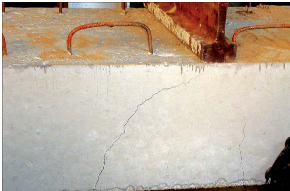
Photo 2 Observed crack patterns at failure for the solid samples (UP 2007)
