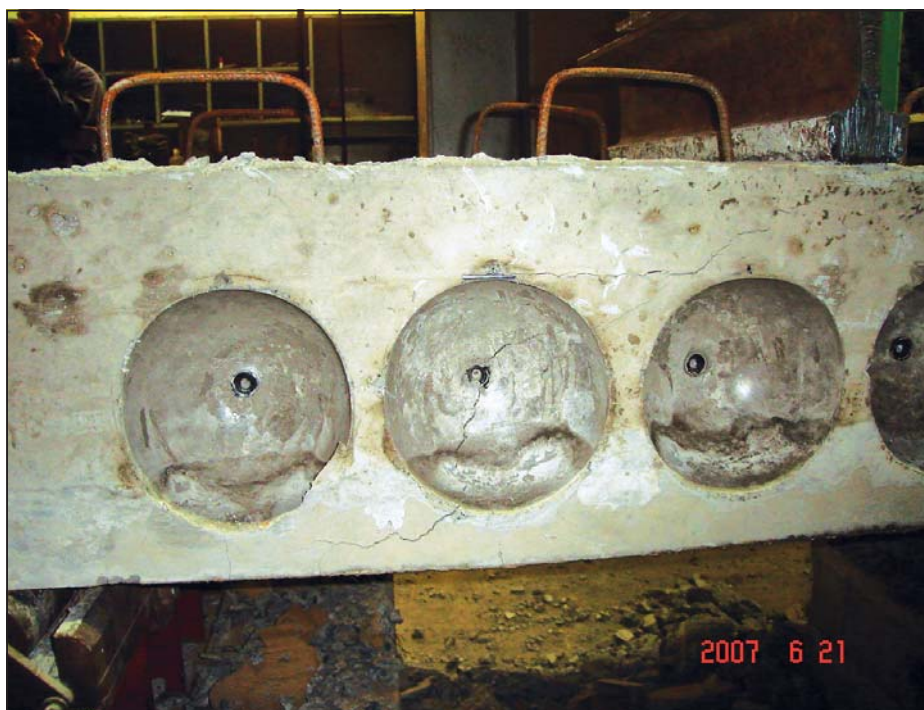
Photo 3 Observed crack patterns at failure for the SVF samples (UP 2007)
