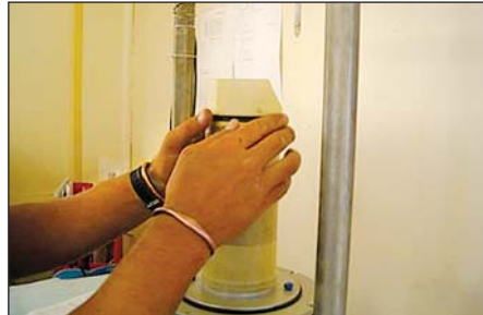
Figure 5 Installing rubber membrane and O-ring seals
