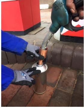
Figure 1: Sampling of fuel from a retail site pump.
