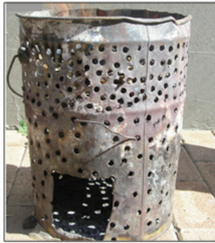
Figure 1. A photograph and schematic representation of a high ventilation field-procured optimised brazier stove used in the experiments (not drawn to scale – dimensions are in mm).
