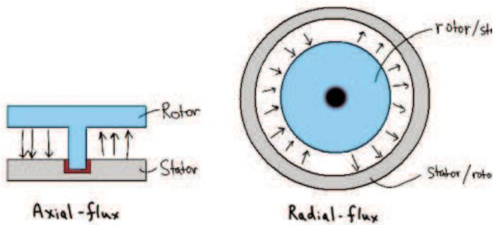
**Figure 5: Cross section of axial and radial flux direction in a typical PMSG, respectively**
