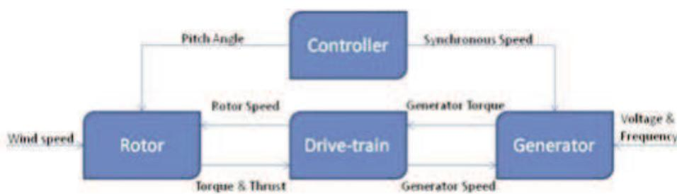
Figure 2: Process flowchart of a typical WEC system
