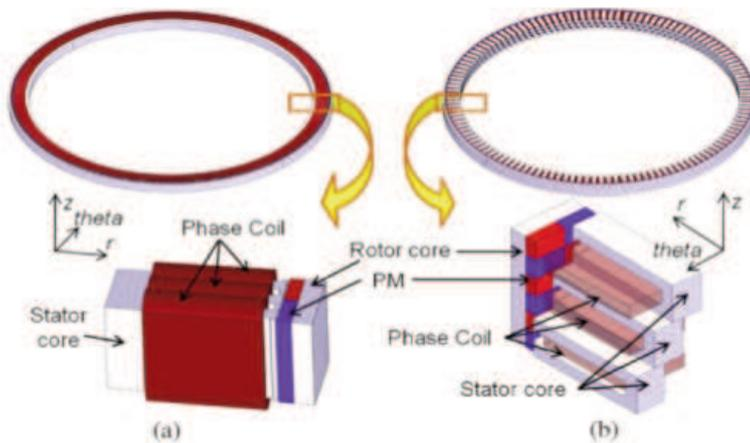
**Figure 6: Cut-out of (a) LFM, (b) TFM**
