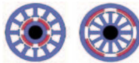
**Figure 7: Internal (left) and external (right) rotor PMSG**
