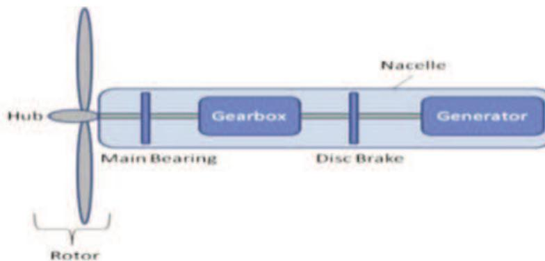
Figure 3: The main parts of a wind turbine
