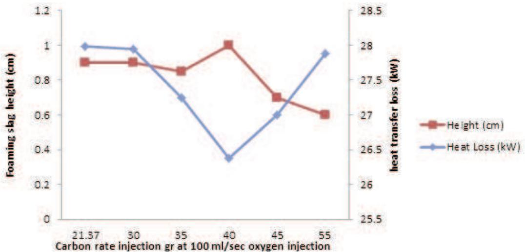
**Figure 19: Comparison and variation of heat transfer (kW) and foaming slag height (cm) due to carbon rate injection at 100 ml/sec oxygen injection**
