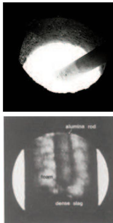
**Figure 7: Overview of the measurement of height of the foaming slag using alumina rod**
