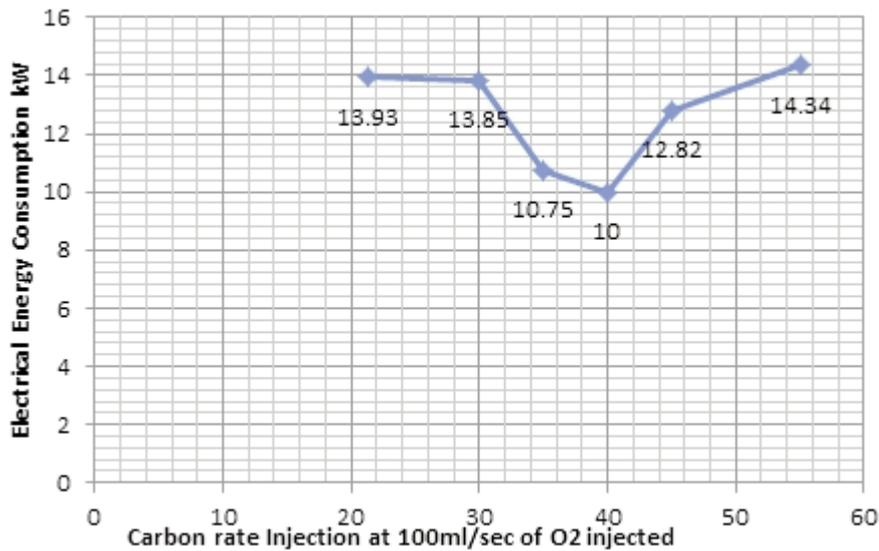
Figure 12: Influence of carbon rate injection on the electrical energy consumption kW
