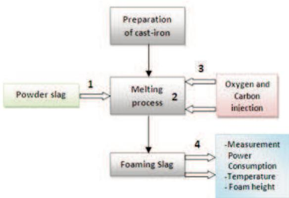
**Figure 6: Schematic diagram of experiment procedure of foaming slag creation**
