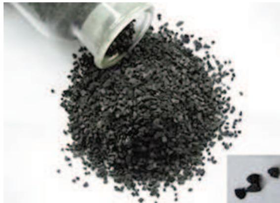
Figure 4: Cast-Iron scraps and carbon particles
