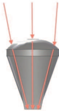
Figure 7: Schematic diagram of the moulded refractive secondary
