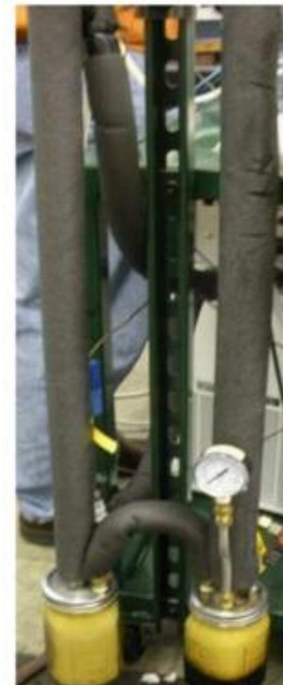
**Figure A3: Bio-oil condensers and containers**
