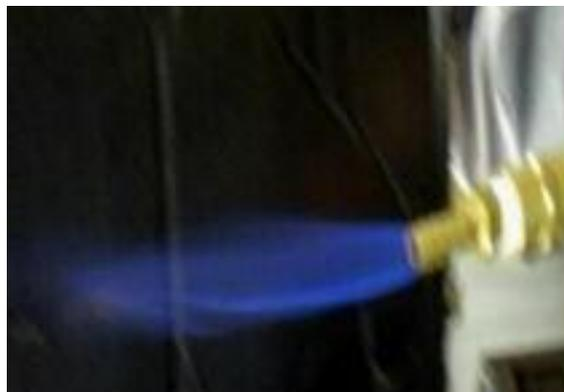
**Figure A5: Combustibility test of NCG**
