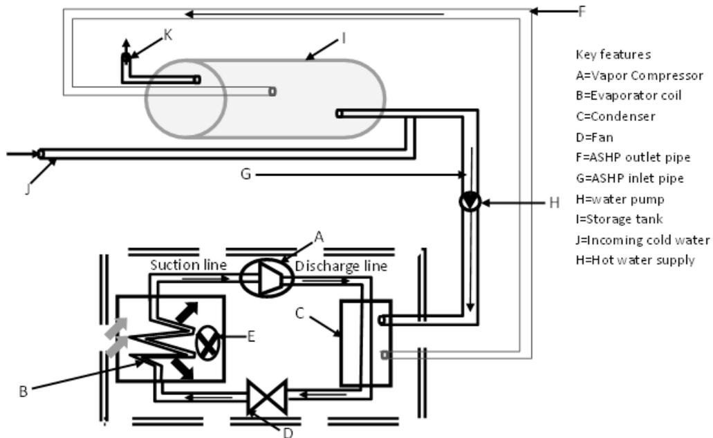
Figure 2: Illustration of an ASHP water heater schematic
