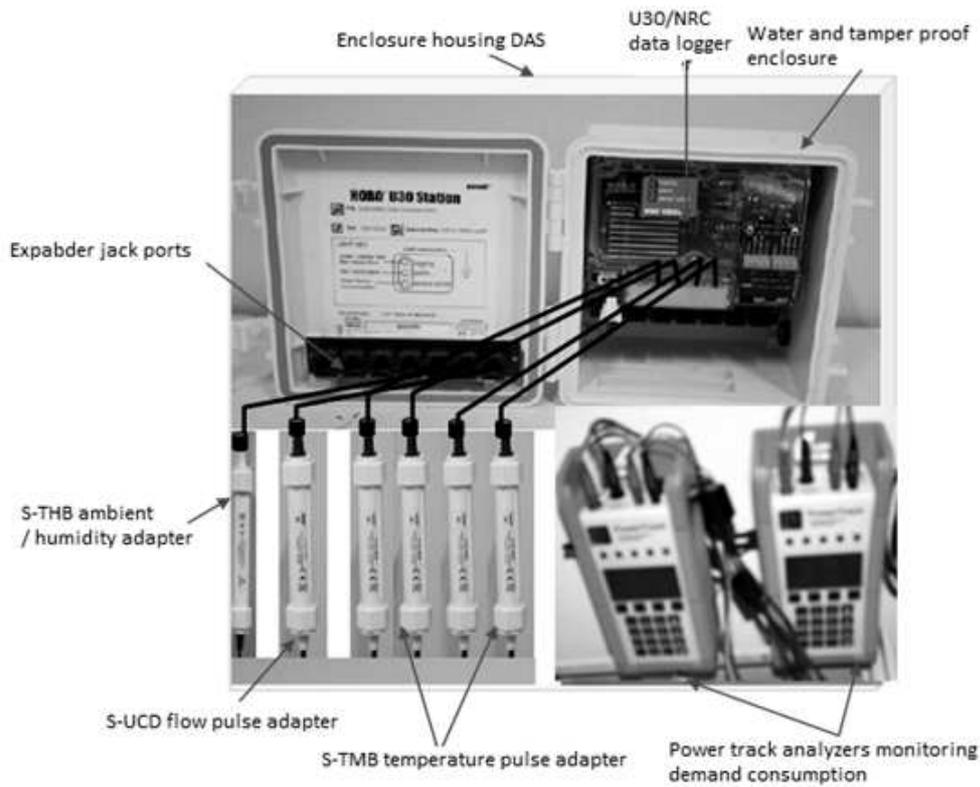
Figure 7: DAS designed and built for the research
