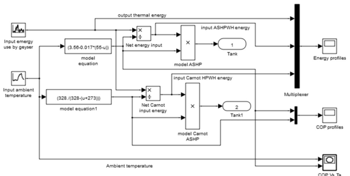
Figure 9: The simulation, architectural and programming sequence used in modelling the system COP and energy consumption
