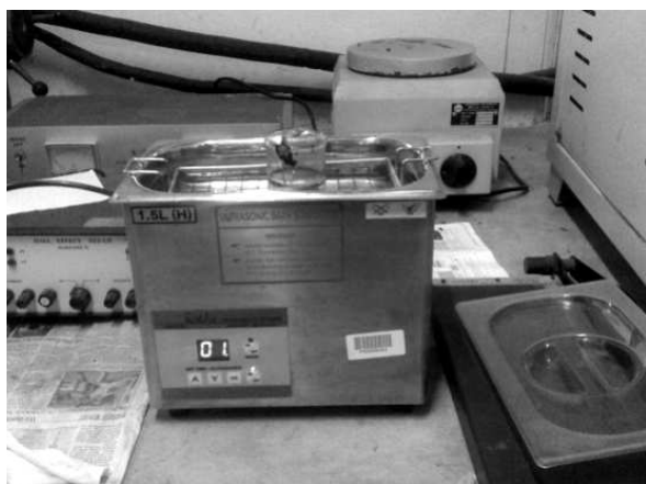
Figure 3: Sonication of nanofluid samples
