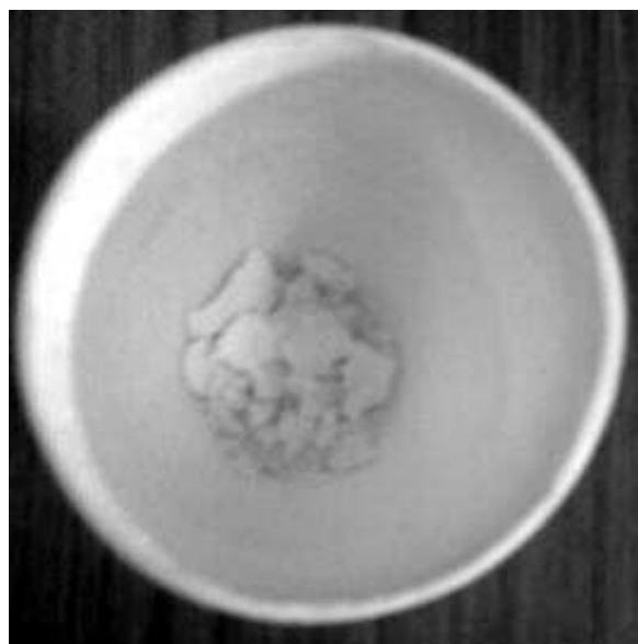
Figure 2: TiO 2 flakes before milling
