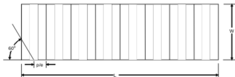
Figure 9: Type and orientation of roughness element investigated by Varun et al. (2008)
