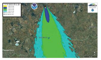
*Figure 7:* HYSPLIT dispersion calculation displayed on a Google Earth map for spontaneous combustion site B for the 23rd of April 2009 (01:00-02:00).
