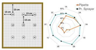
**Figure 2:** Spatial variation test to verify and optimize nanoparticle deposition uniformity. The spider-chart depicts the uniformity of the pressurized sprayer over the pipette deposition.
