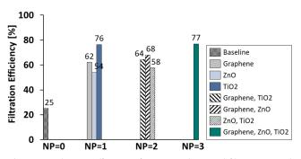
**Figure 12:** Filtration efficiency of nanoparticle coated filters improved significantly relative to a baseline uncoated filter. The Graphene, ZnO, TiO, combination is 3 times more effective than a baseline uncoated filter.
