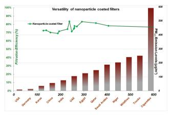
**Figure 14:** Versatility of nanoparticle coated filters in different global pollution levels. The bar-chart indicates the different  $PM_{25}$  levels in different countries and from different sources. The line graph indicates the filtration efficiency relative to the inlet  $PM_{25}$  levels, indicating relatively consistent filtration efficiency over a wide range of  $PM_{25}$  levels (100~600  $\mu g/m^3$ ).
