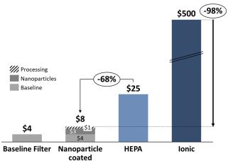
**Figure 13:** Adding the costs of the nanoparticles and processing costs to a baseline filter, the coated filters are significantly less expensive than HEPA or ionic filtration systems.
