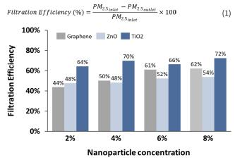
**Figure 7:** Increase in nanoparticle concentration improves filtration efficiency. TiO<sub>2</sub> has the overall highest filtration efficiency, while Graphene demonstrates the strongest correlation in filtration efficiency and concentration.
