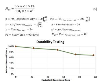
Figure 11: Relative filtration efficiency maintained up to 90% of the initial efficiency during accelerated durability testing over 50 equivalent days.
