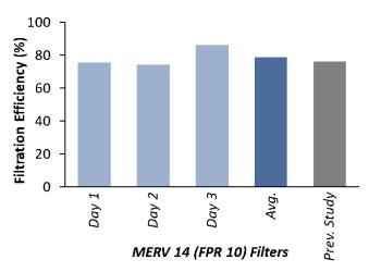
**Figure 5:** Commercially available MERV14 filters' filtration efficiency was maintained over different days of testing and was found to be consistent to a previous study, thus confirming the validity of the experimental setup.
