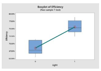
Figure 9: A 2-sample t-test demonstrating impact of light on filtration efficiency of TiO.
