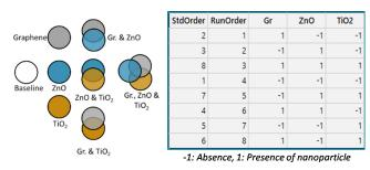
**Figure 4:** Design of Experiments set-up using full-factorial design for ANOVA analysis. The table indicates the run order used to randomize the experimentation to avoid bias. The figure on the right illustrates the different combinations of the nanomaterials used for the experiment.
