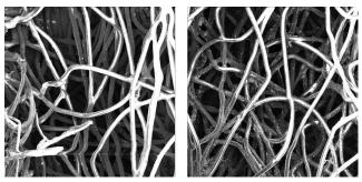
**Figure 3a:** Scanning Electron Microscope (SEM) images of the baseline filter (left) and the TiO<sub>2</sub> coated one (right) confirm the adhesion of the nanoparticles to the fibres of the filtration media.
