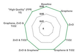
Figure 10: Nanoparticle coated filters have no measurable impact on the pressure drop.
