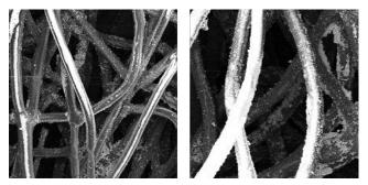
**Figure 3b:** Scanning Electron Microscope (SEM) images of the  $TiO_2$  coated filter before (left) and after (right) exposure to  $PM_{2.5}$  particles, show the adsorption of the  $PM_{2.5}$  particles to the nanoparticle adhesion areas of the filtration media.
