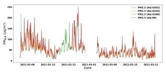
**Figure 4:** Comparison between hourly PM<sub>2.5</sub> values between AirQo devices collocated at Makerere University
