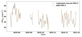
Figure 2:  $PM_{25}$  comparisons for AirQo device AQ88 vs BAM collocated at Makerere University
