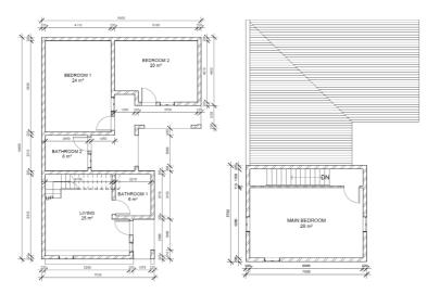
Figure 4: K206 Housing unit first-floor plans Source: Adapted from Osman & Davey, 2011: 7
