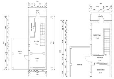
Figure 5: A 10X10 Sandbag House floor plans Source: Adapted from Johnson, 2014: online
