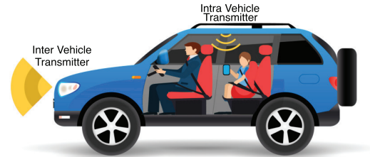
Fig. 2: VLC system for both intra- and inter-vehicle communication 1
