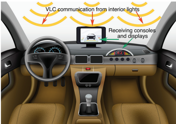
Fig. 4: VLC system for intra-vehicle communication 1
