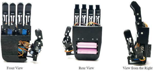
Fig. 6: The working prototype of the hand. Pay special attention to the palm and how everything, except the batteries are located inside the palm.
