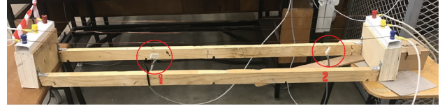
Fig. 4. Scaled power line showing sensor positions.
