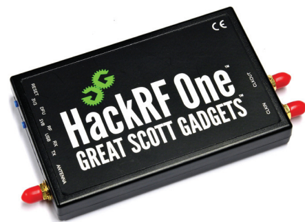
Figure 4: A HackRF One SDR.
