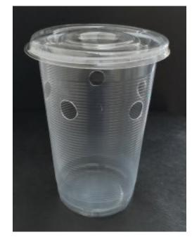
**Figure 2.** Deli cup trap constructed from transparent 370 ml disposable cup (Everpack, Accra, Ghana) by drilling five holes (diameter ~12 mm) equidistant to each other and ~3 cm from the top of the cup
